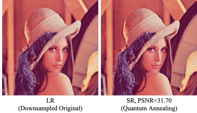
Figure 5. Result on the full Lenna image using the Quantum Annealing algorithm with a magnification factor of 3. Left: LR. Right: SR using Quantum Annealing.
